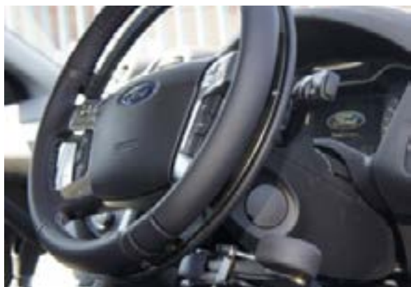
Examples of push-pat hand controls and under-ring, over-ring and thumb operated accelerators with hand operated brakes
