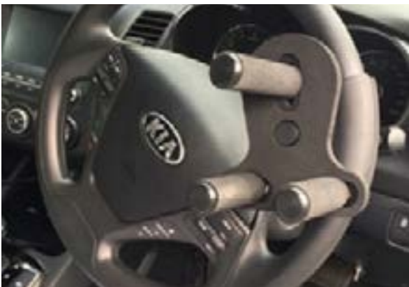
Different examples of steering devices +/- integrated secondary controls
