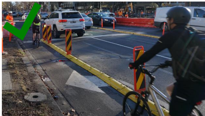
FIGURE 27: DELINEATION OF CYCLISTS FROM TRAFFIC LANE
