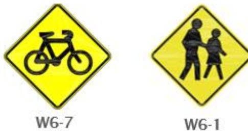
FIGURE 29: PEDESTRIAN AND CYCLIST WARNING SIGNS
