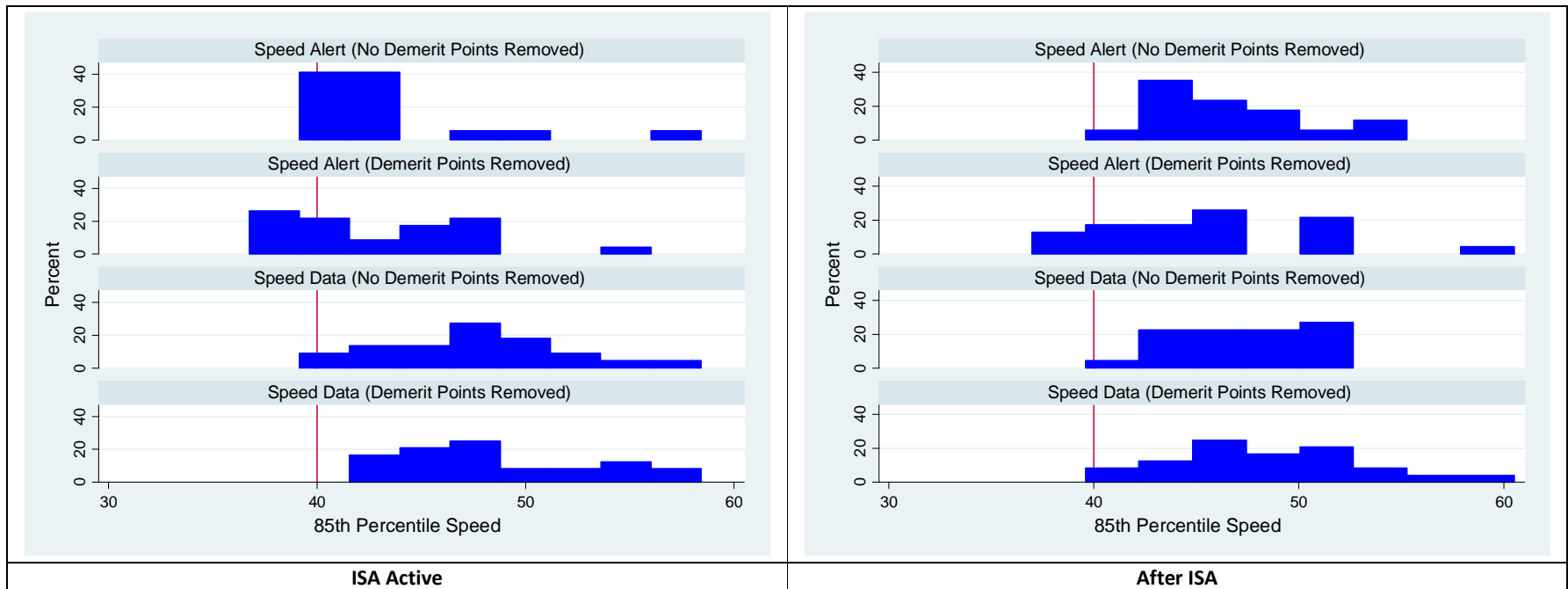
Figure F.13 Distribution of 85th percentile speed for 40 km/h speed zones
