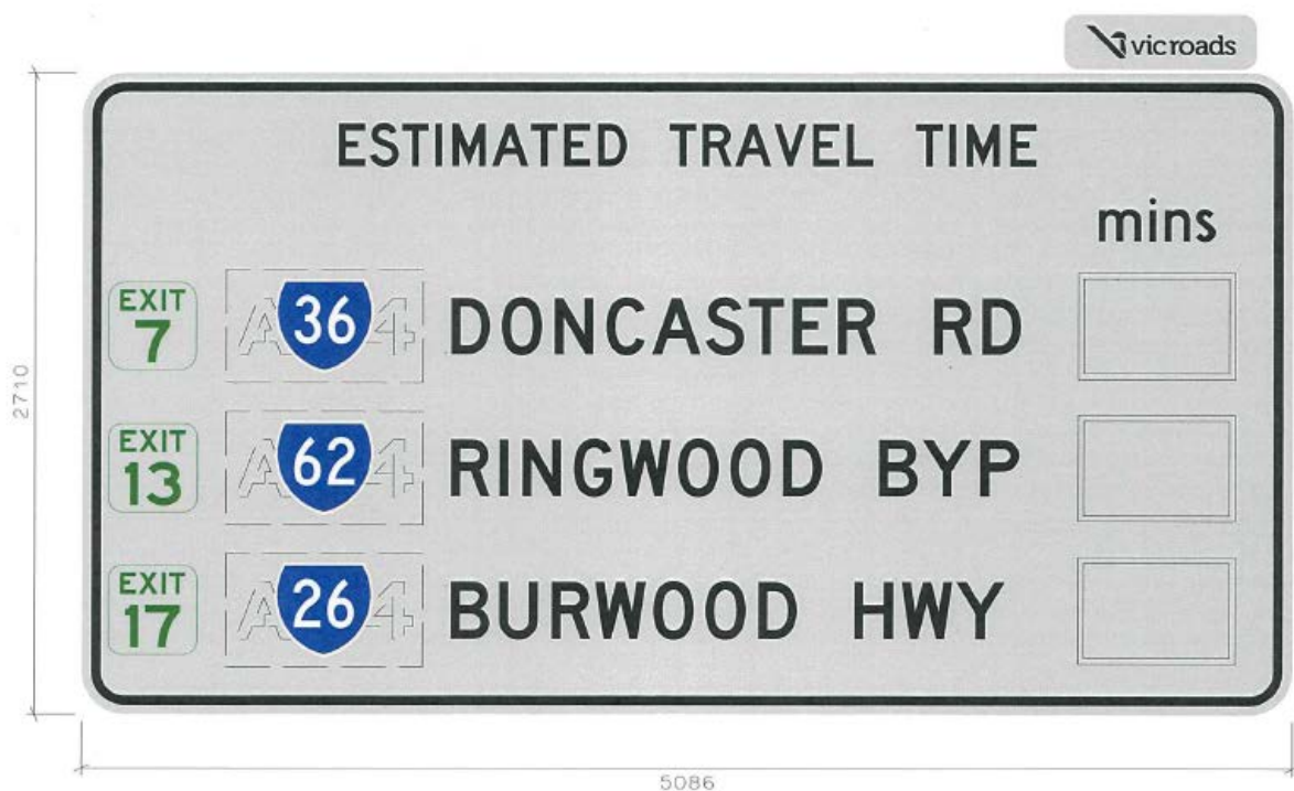
FigureE.1 - Typical Layout for C Size sign on Freeway
