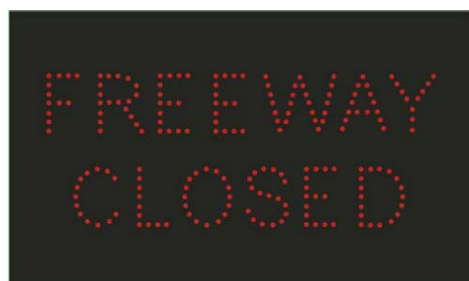
Figure 3.2 – Typical layout for FREEWAY CLOSED display for Ramp Control Operation (Provided as examples only)
