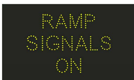
Figure 3.1 – Typical layout for RAMP SIGNALS ON display for Ramp Metering Operation (Provided as an example only)
