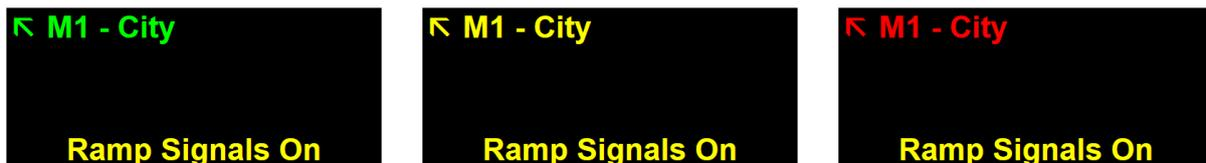
Figure 7-13: Typical 'Ramp Signals On' displays – single direction ramp
