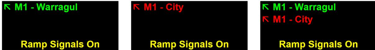
Figure 7-14: Typical 'Ramp Signals On' displays – two-direction ramp
