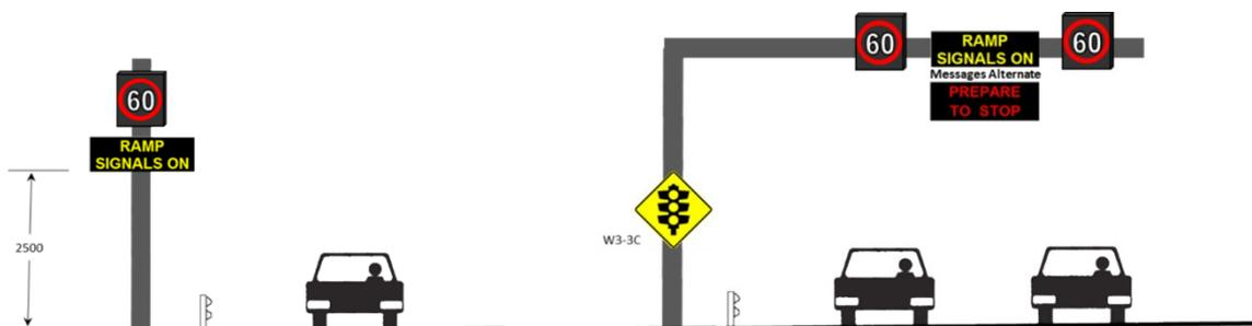
**Note:** RAMP SIGNALS ON (yellow) alternates with PREPARE TO STOP (red)
