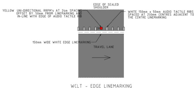
Red Raised Reflective Pavement Markers (RRPM's) are placed offset by 50mm from the edge of the linemarking. The outside edge of the RRPM should be aligned with the outside edge of the audio tactile rib. RRPM's are to be placed at 24m spacing.
