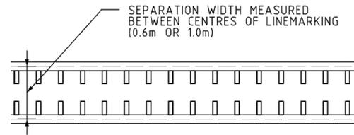
Figure 2.1.2 WCLT Separation Width
