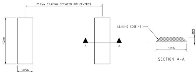
White audio tactile ribs are used for WCLT by TMR in Queensland and Main Roads WA and should be used in Victoria for consistency. White audio tactile ribs with these dimensions and spacing is consistent with the 2018 Austroads harmonisation project for pavement marking<sup>6</sup>.
