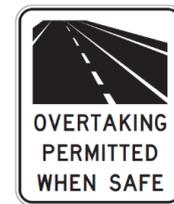
Double One-Way Barrier Line Marking Sign Permitting Overtaking
