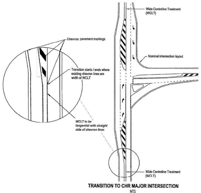
Figure 4.5.1 - Figure F.2 WCLT at channelised right turn intersections
