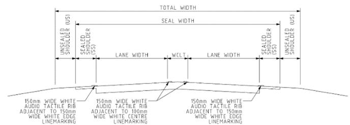
Figure 4.2 Wide Centre Line Treatment Typical Cross Section
