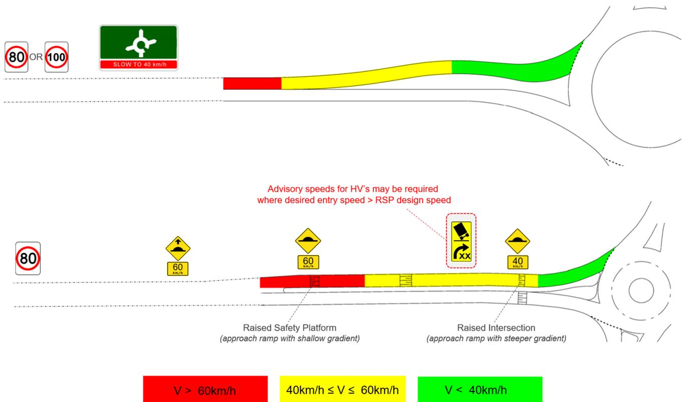
**Figure 4: Visualisation of speed reduction logic on the approach to a conventional (top) and compact (bottom) roundabout (not to scale and not all signage shown)**
