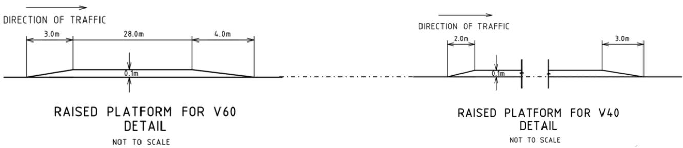
**Figure 21: Lance Creek raised safety platform profiles**
