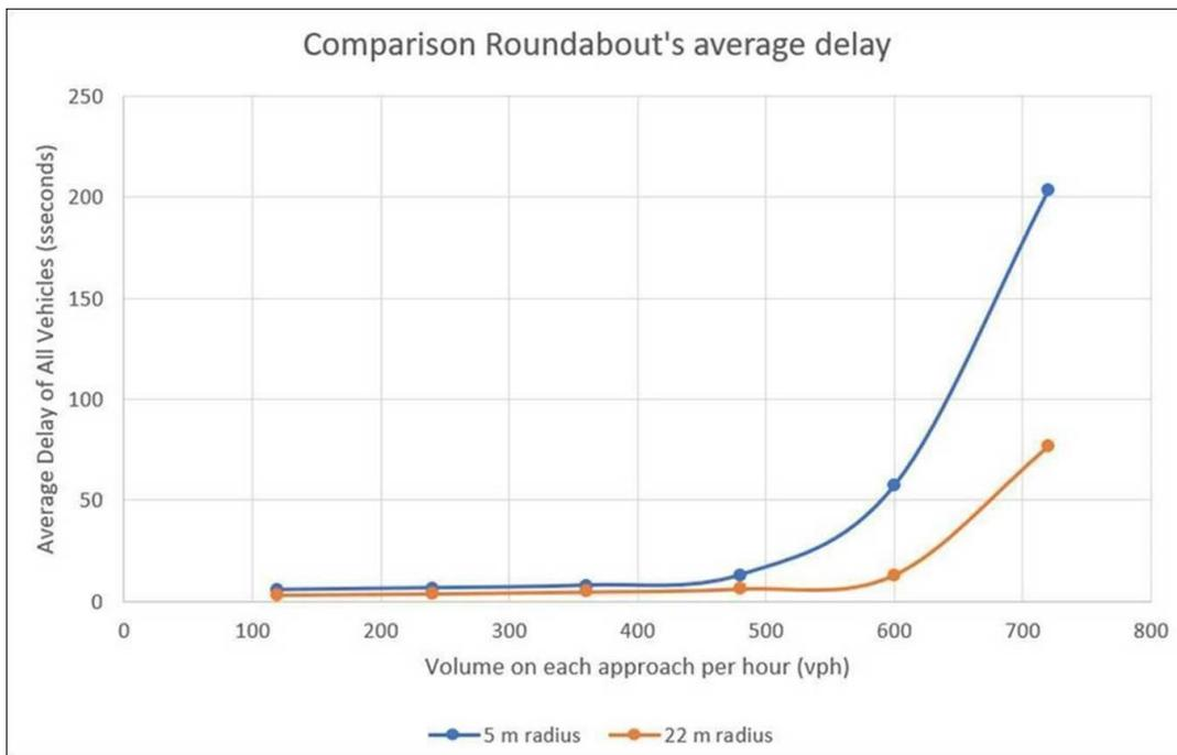
**Figure 23: Delays caused by compact and conventional roundabouts**
