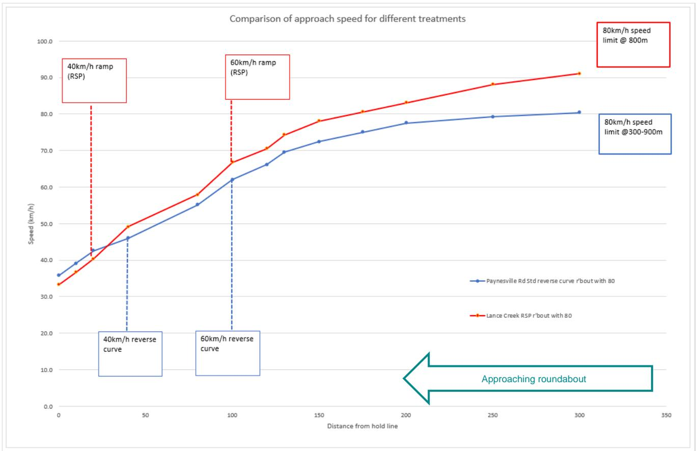
**Figure 20: Comparison of approach speed by distance for reverse curve and raised safety platform**
