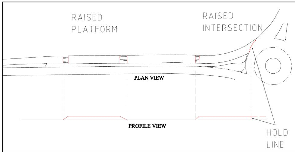
**Figure 5: Profile of a compact roundabout with a raised intersection (not to scale)**
