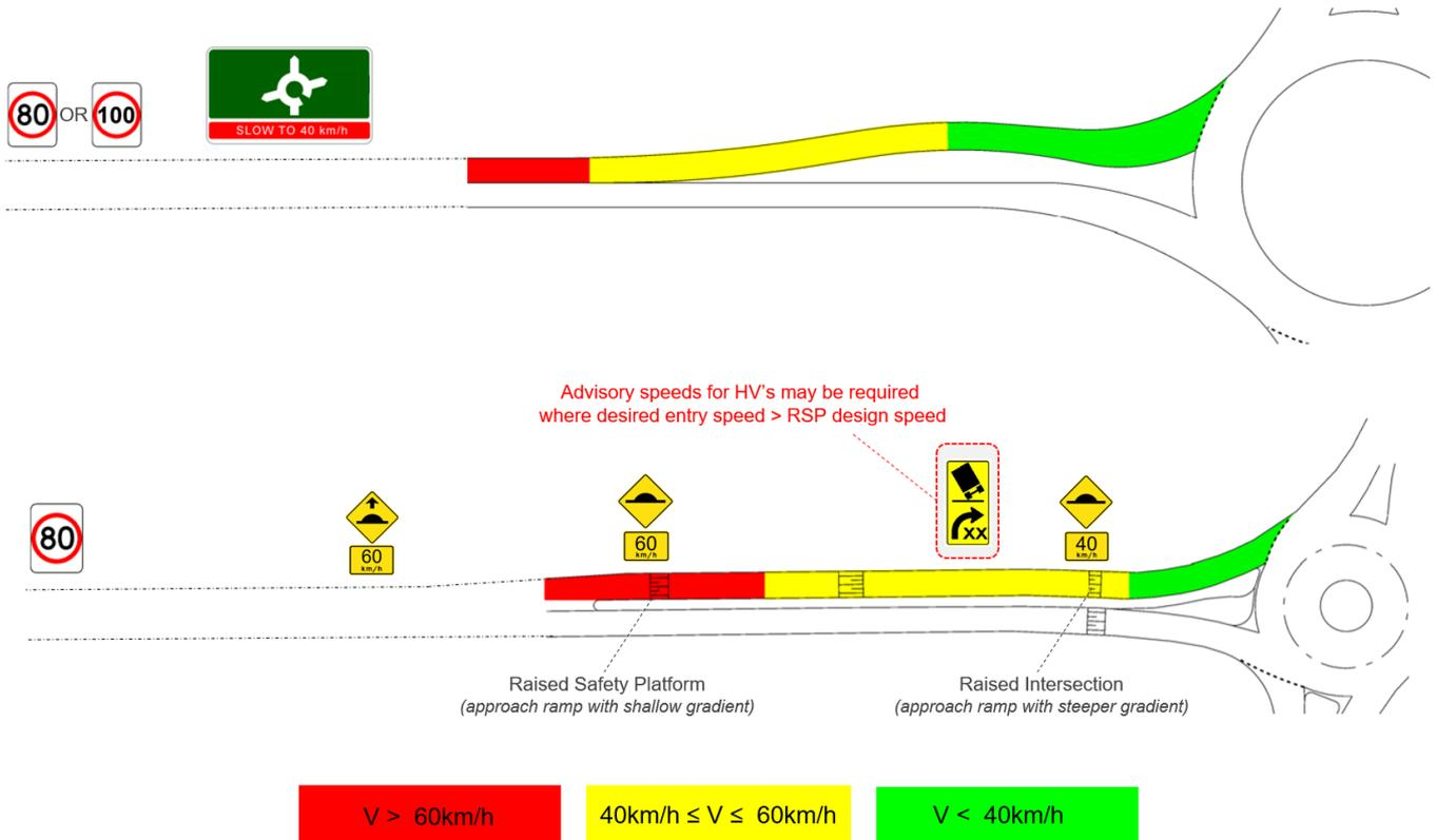
**Figure 19: Visualisation of speed reduction on the approach to a compact (top) and conventional (bottom) roundabout (not to scale and not all signage shown)**
