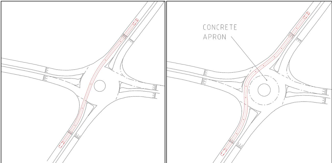
**Figure 9: a. operation with wide carriageway, b. operation with concrete apron – movement deflection**
