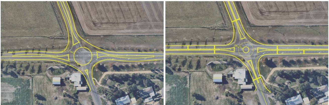
**Figure 13: Example concept designs for a conventional and compact roundabout**
