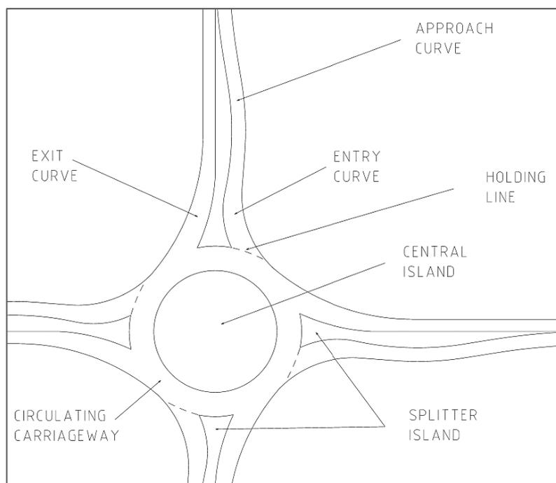
**Figure 2: Important Components of Conventional Roundabouts**
