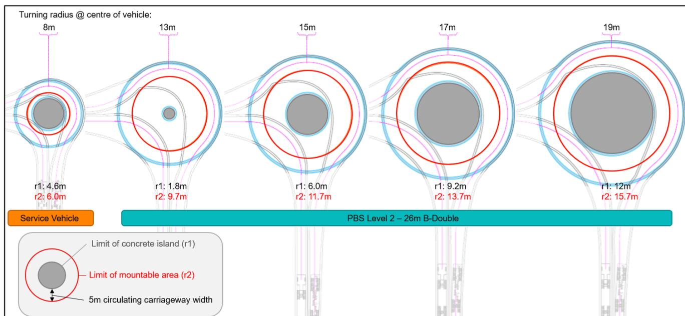
**Figure 8: Impact of design vehicles turning radii upon size of concrete island & mountable area**
