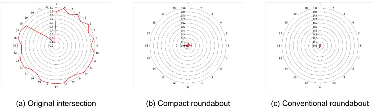
**Figure 15: a) FSI Probability - Original Intersection (100 km/h), b) FSI Probability - Compact Roundabout (80 km/h), c) FSI Probability - Conventional Roundabout at Paynesville Road (80 km/h)**
