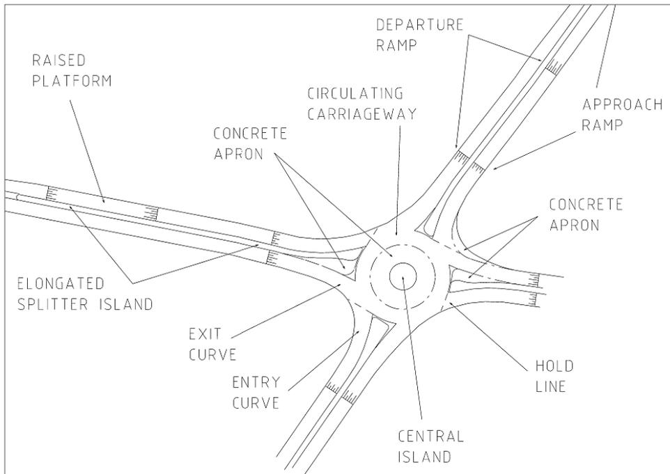
**Figure 1: Important Components of Typical Compact Roundabouts**
