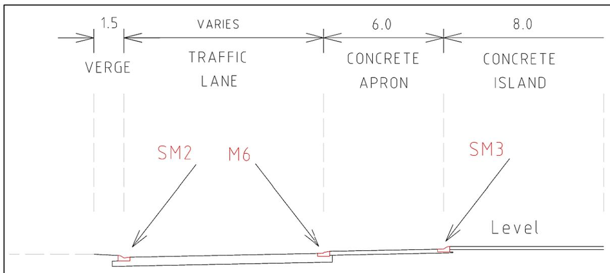
**Figure 11: Kerbing adopted at the Lance Creek roundabout**
