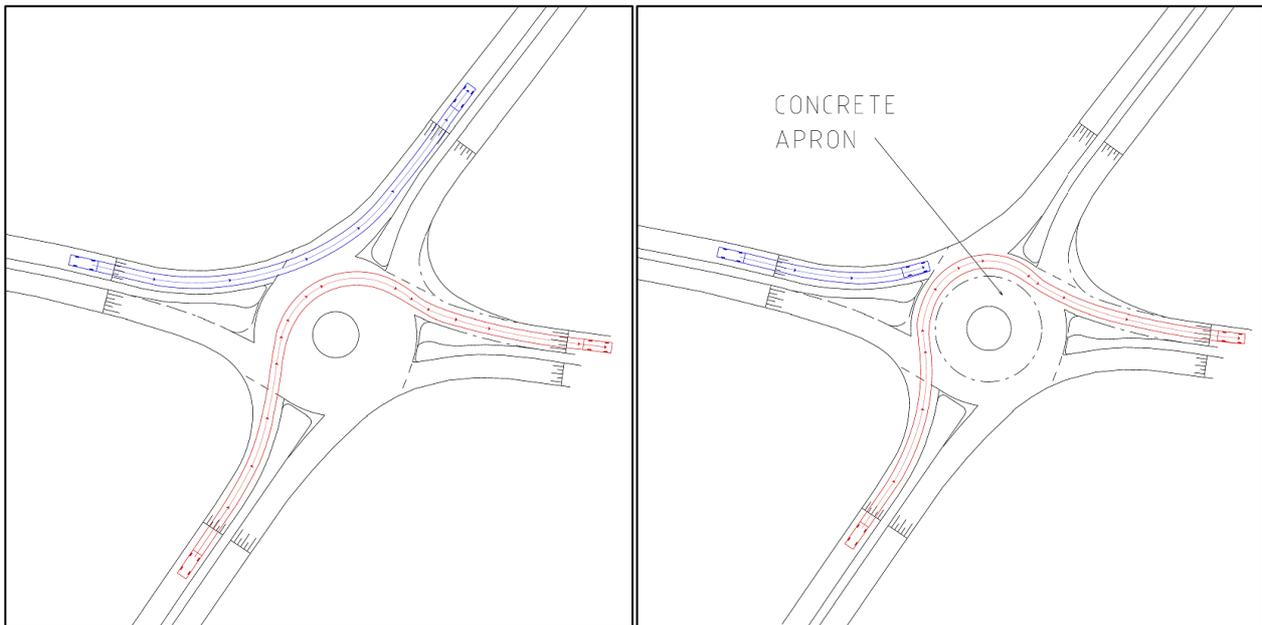
**Figure 10: a. operation with wide carriageway, b. operation with concrete apron.**
