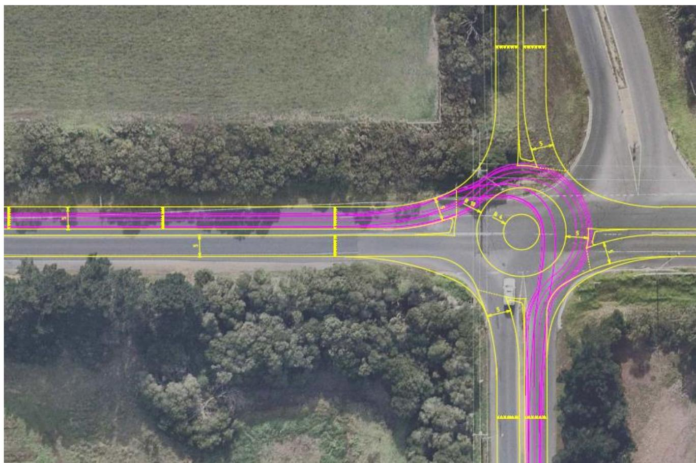
**Figure 12: Swept path of a B-Double during the design of a compact roundabout**
