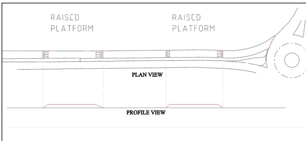
**Figure 6: Profile of a compact roundabout without a raised intersection (not to scale)**
