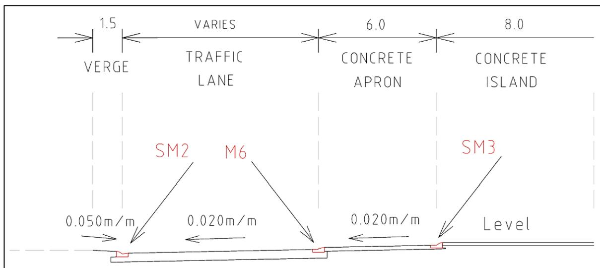
**Figure 16: Grading of roundabout cross section**
