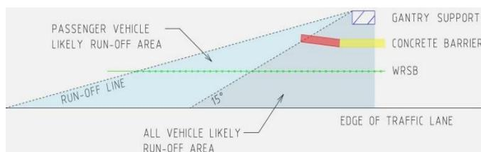
Figure 6.6: Two-stage protection points of need
