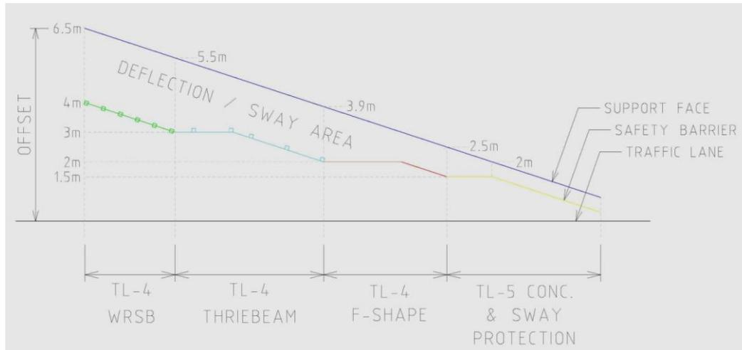
Figure 6.2: Example of TL-4 barrier type vs. offset
