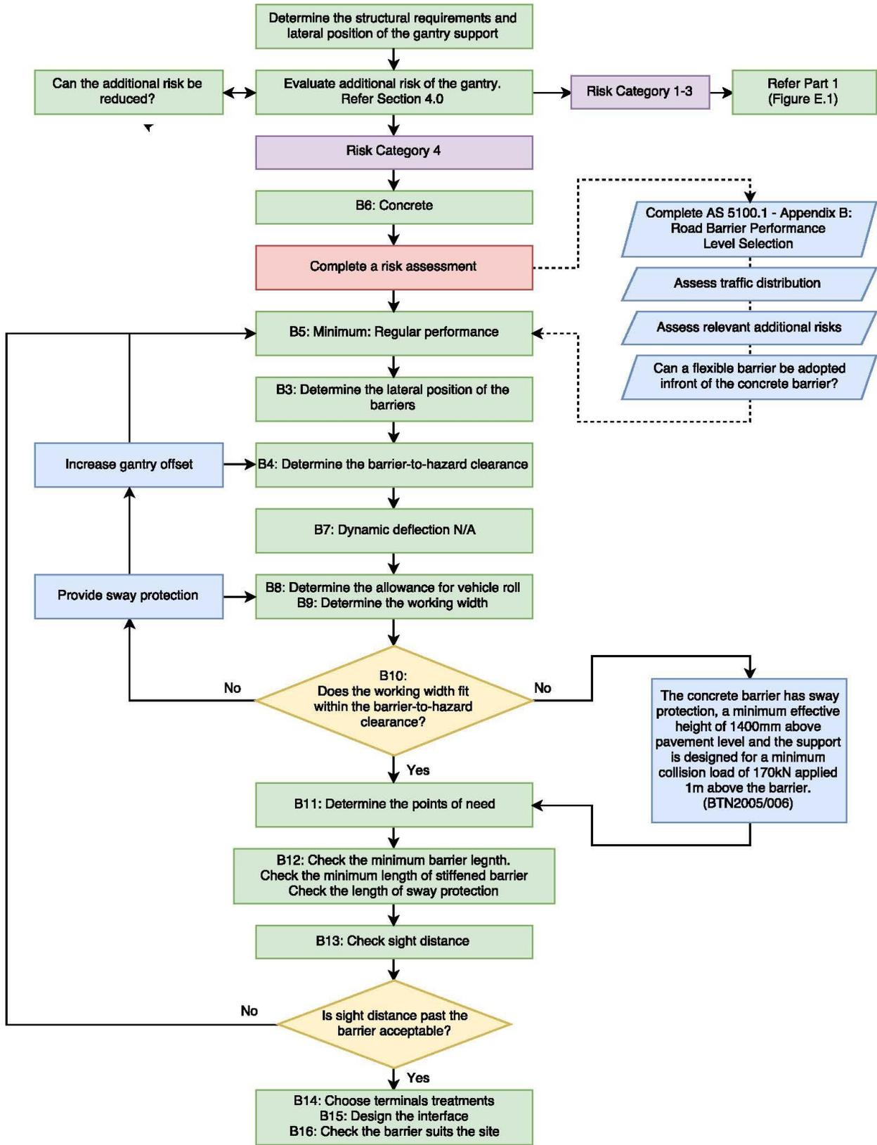
Figure F.2: Modified road safety barrier design process for the protection of gantry and cantilever sign supports (Part 2) (Original Source: Source: AGRD Part 6, Figure 6.1)
