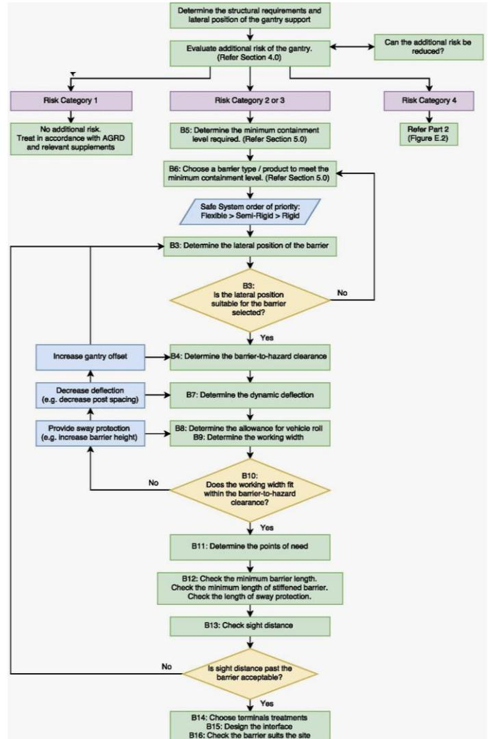
Figure 6.1: Road Safety Design Process (Modified) (Source: Appendix E, Figure E1)
