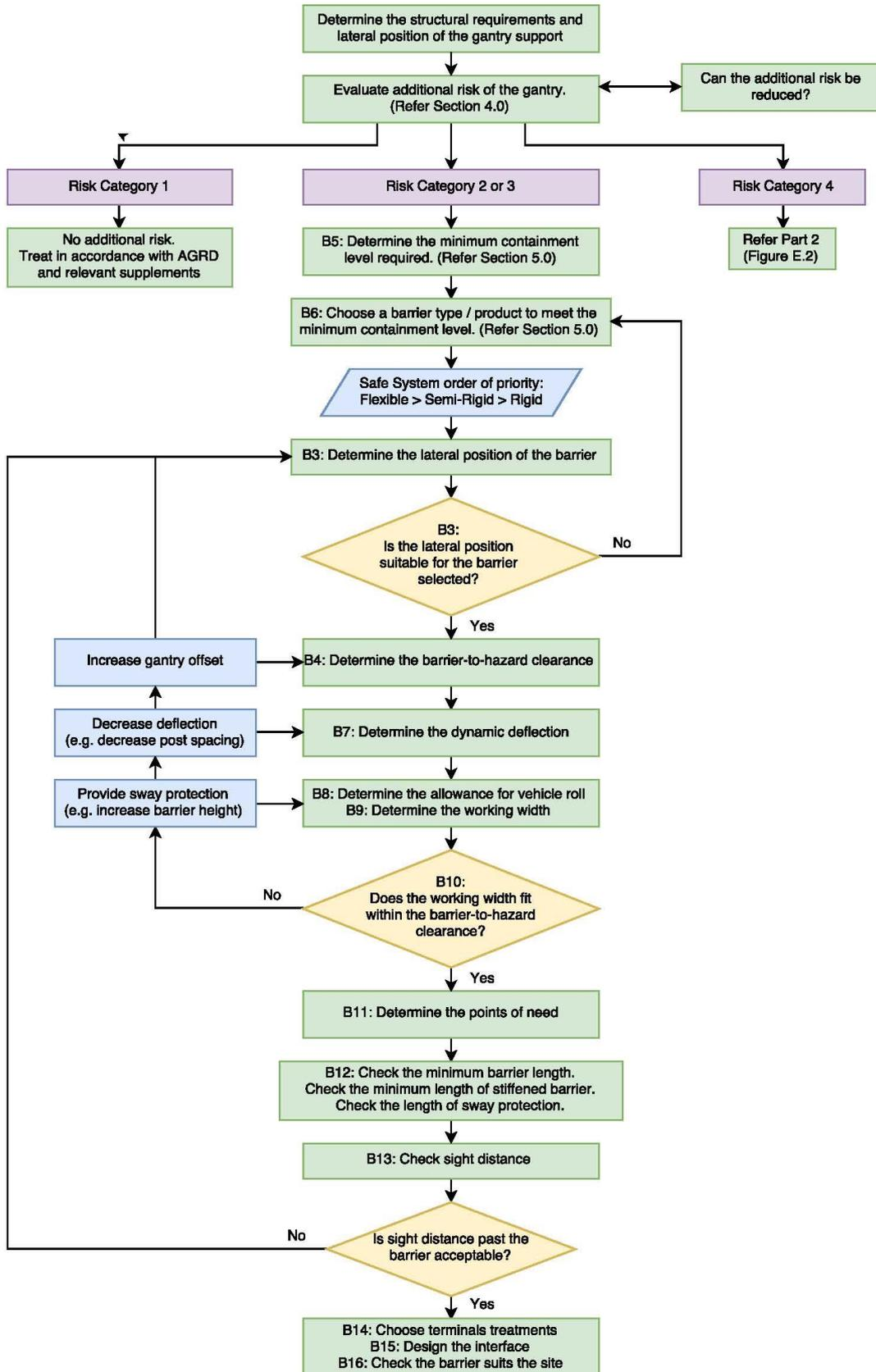
Figure F.1: Modified road safety barrier design process for the protection of gantry and cantilever sign supports (Part 1) (Original Source: Source: AGRD Part 6, Figure 6.1)
