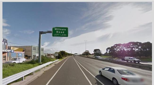
This cantilever support projects over a single on-ramp traffic lane. Thriebeam is TL-4 and is unlikely to be penetrated. In the event of a collapse, vehicles are unlikely to be impacted and the structure would have minor disruption to the network until repaired.
