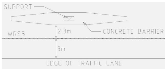
Figure 7.1: Example of two-stage protection
