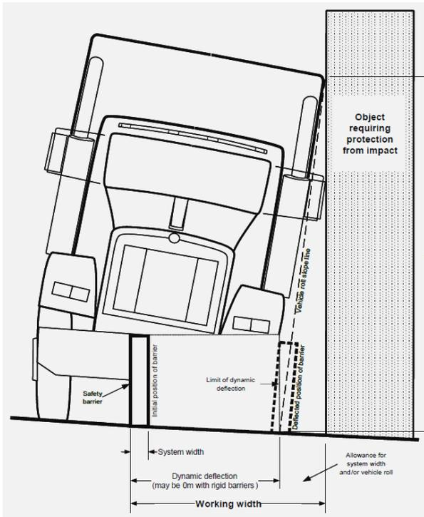
Figure 6.3: Working Width
