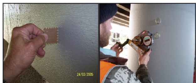
Fig. 5 Wet Film Thickness Gauge (L), Dollies attached onto coating surface and pull-off test in progress (R)
