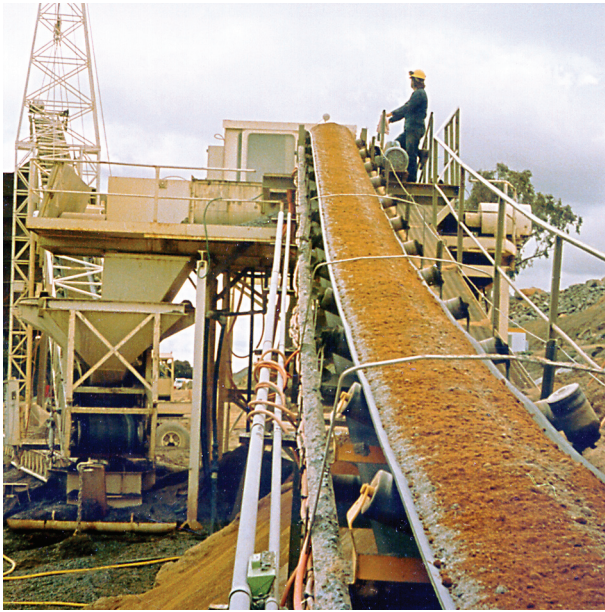
Crushed rock with clayey sand additive prior to pug-milling
