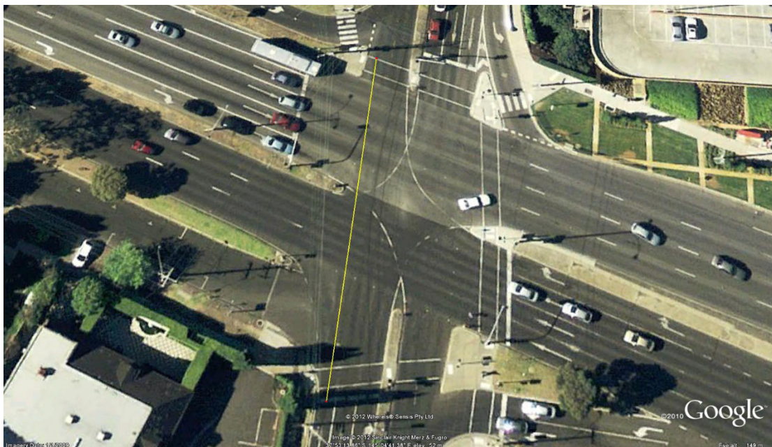
Figure 1: Through movement, measure from stop line to far side of pedestrian crossing
