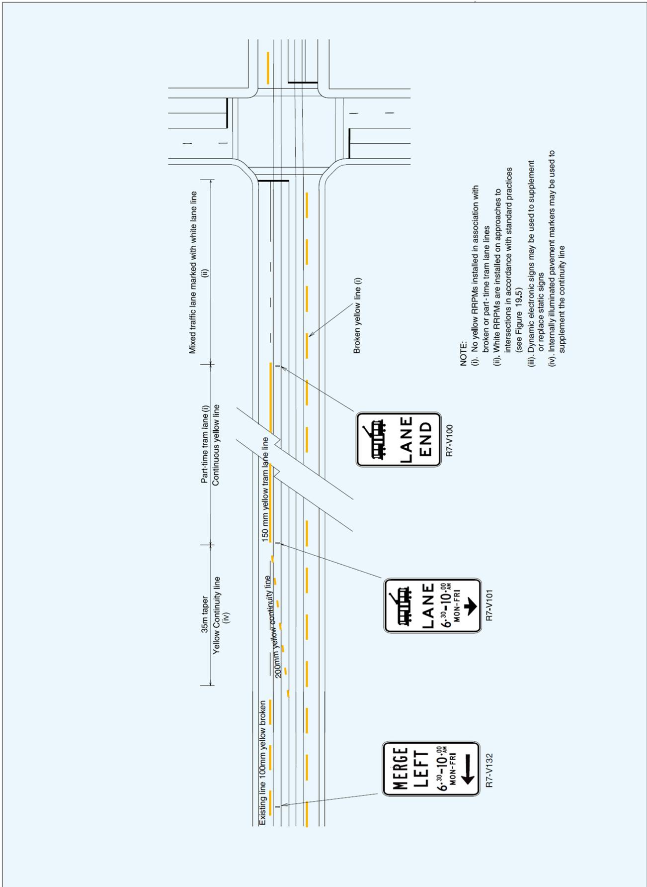
Figure 9: Typical layout of part-time tram lane on a four-lane undivided road
