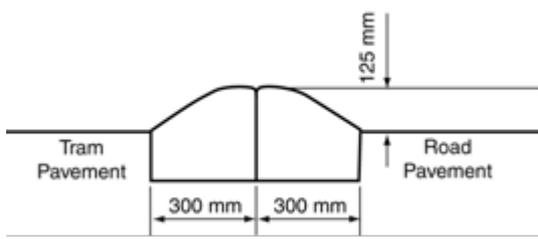
**Figure 12: Semi mounted kerb profiles**
