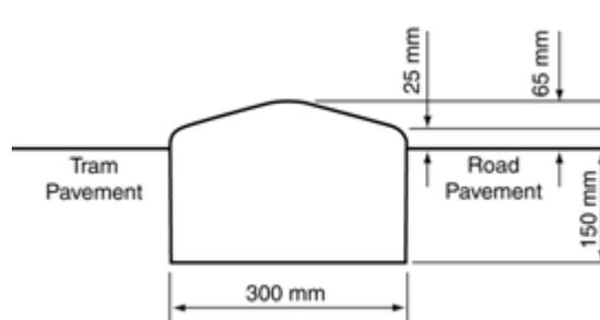
Figure 11: Low profile concrete kerbing
