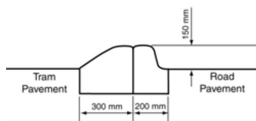
**Figure 13: Barrier and semi mountable kerbs**
