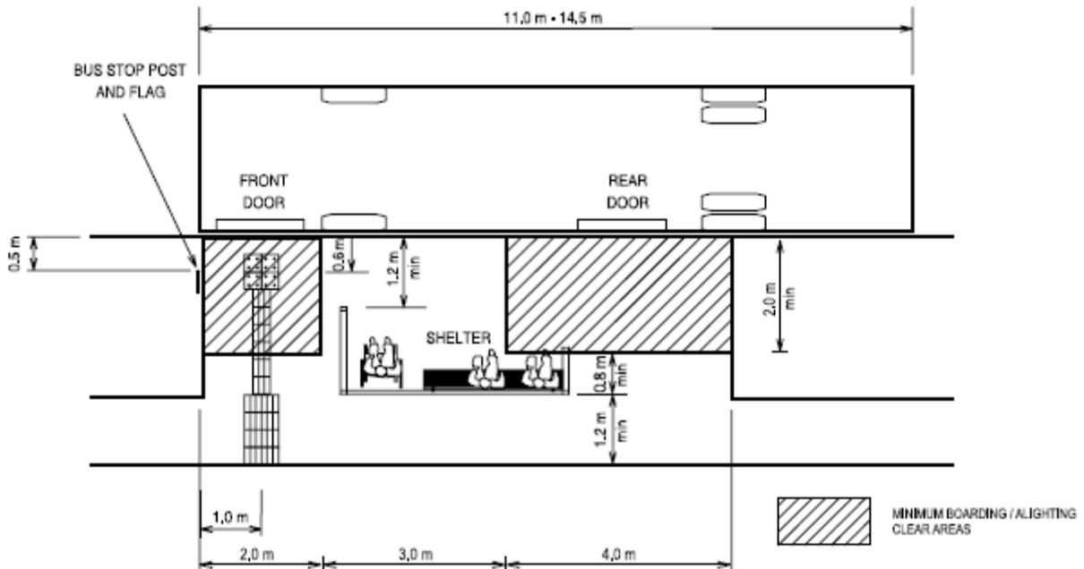
**Figure 14: Preferred bus stop layout – roadside width > 3.2m (with 3m long shelter) or > 4.0m (with larger shelter as shown)**
