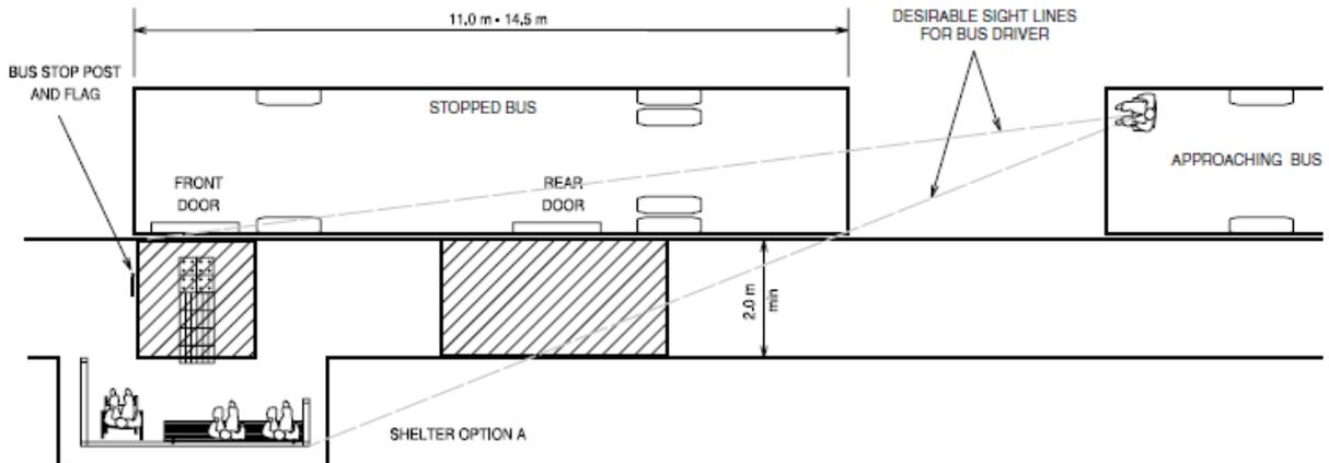
**Figure 15: Bus passenger shelter location option A – roadside width >2.0 m**
