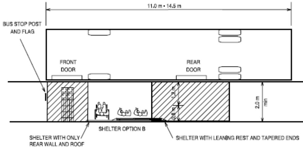
**Figure 16: Bus passenger shelter location option B – roadside width >2.0 m**
