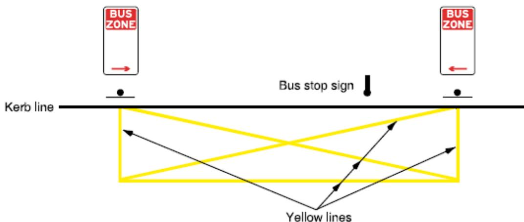
**Figure 18: Bus Zone sign and Bus Zone pavement markings**
