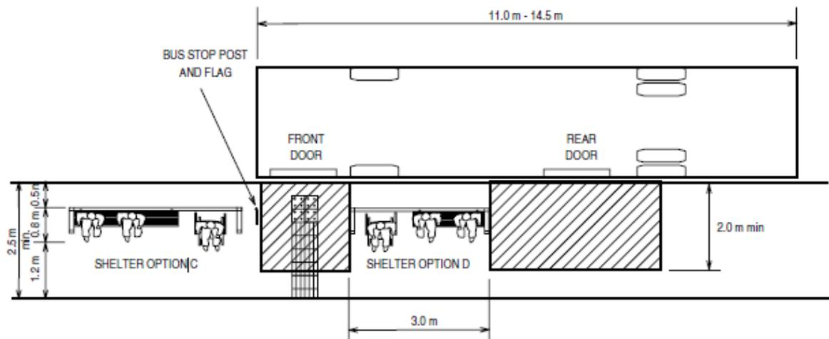
**Figure 17: Bus passenger shelter location options C and D – roadside width >2.5 m**
