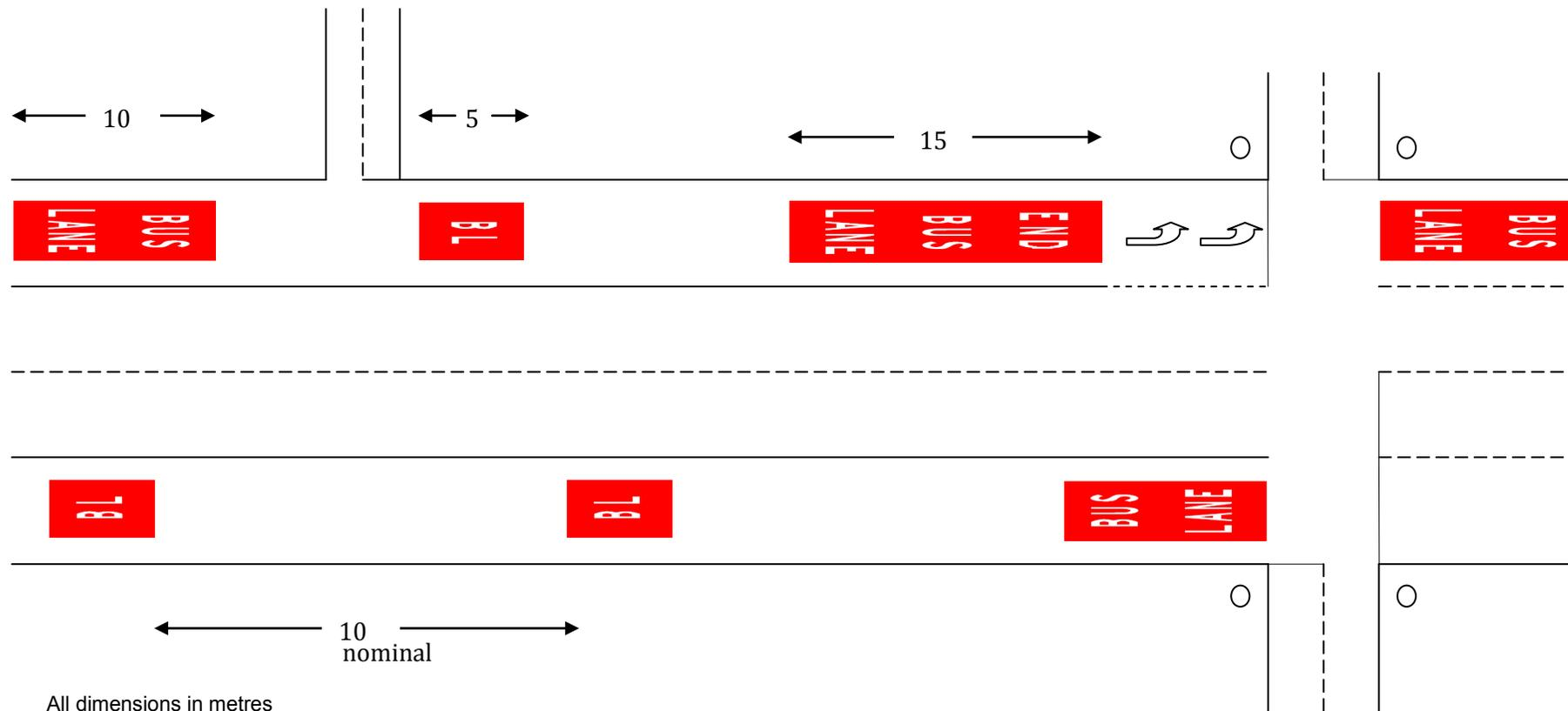
**Figure 4: Example of red colour patch Bus Lane markings**
