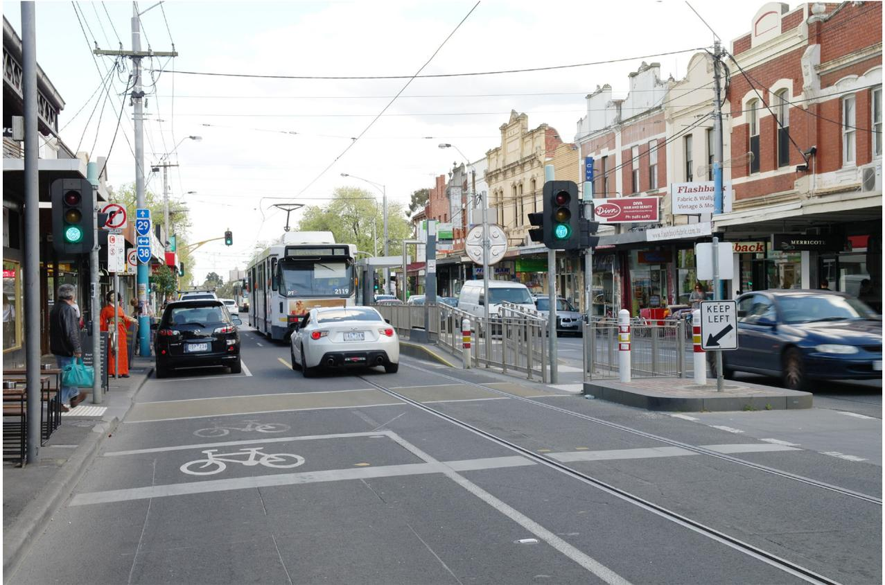
**Figure 25: Centre island platform stop, vehicles permitted adjacent to tram tracks (during Clearway times) – High St / Westgarth St, Northcote**
