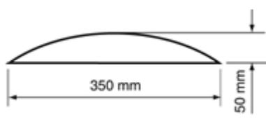
Figure 10: Rubber kerbing profile
