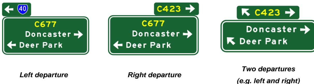
**Figure 47: Installation location for top knots**
