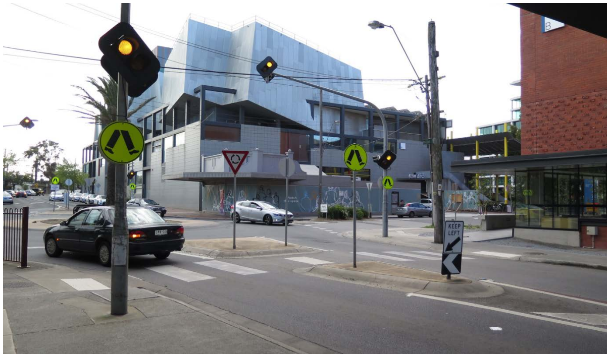
Figure 41: Pedestrian crossing at Sir John Monash Drive / Queens Avenue, Caulfield, with a setback to store vehicles between the crossing and roundabout.
