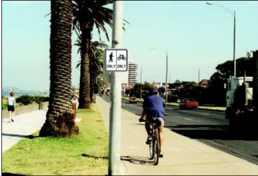
Figure 38: Example of separated pedestrian and cyclist path
