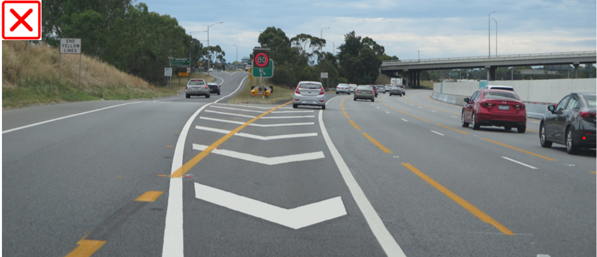
Figure 3: Example of remnant white markings potentially leading to confusion
