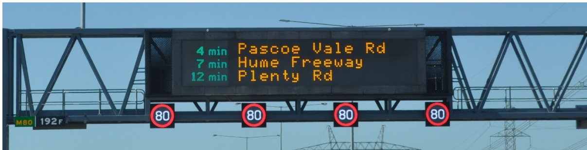
Figure 8-2: Composite VMS signs showing trip condition and travel time information.
